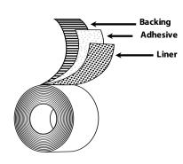
Backing:1/32" white, crosslinked polyethylene foamAdhesive:Non-Sensitizing Acrylic (M108)Liner:74lb bleached polycoated kraft, silicone<br/>treated on one side
