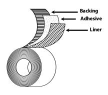
Backing:1/8" white, crosslinked polyethylene<br/>foamAdhesive:Non-irritating acrylic (M111)Liner:2 mil clear BOPP film, silicone treated on
